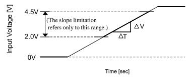
Slope :  $S = \Delta V / \Delta T$  [V/sec] S :  $\frac{1V}{20us}$  to  $\frac{1V}{20ms}$
